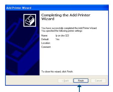
The wizard will install the printer drivers, and return a completion screen. Click **Finish**.
